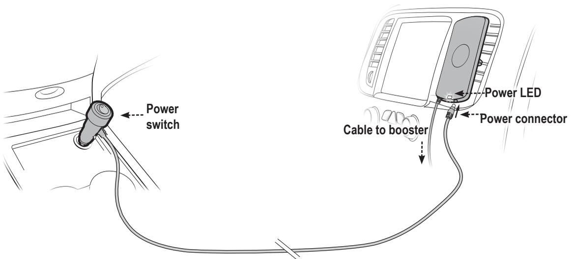
**WARNING:** The booster is rated for 5-15V input voltage. DO NOT use the booster with a higher voltage power supply. This can damage the booster and/or cause personal injury.
