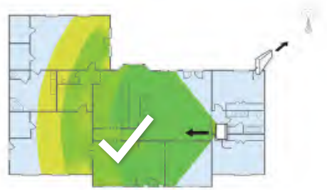
Face inside antenna away from outside antenna
