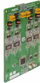
The 4-Port CO Line Card with Caller ID is an expansion card that provides four additional CO line ports with built-in Caller ID. You can install this card only in the bottom expansion slot for a system maximum of 8 outside line ports.
