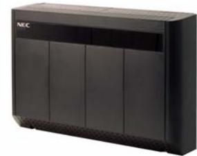
The DSX-160 8-Slot KSU contains the CPU slot, 8 universal card slots and up to 3 system power supplies (depending on Load Factor requirements). It provides 160 ports. Just like the DSX-80 4-Slot KSU, the DSX-160 is wall-mountable, has a flip off cover and removable side panel for easy access. The DSX-160 also has a translucent panel in the cover for getting essential system status and troubleshooting at a glance.
