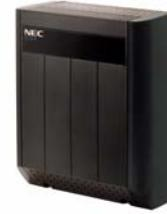
The DSX-80 4-Slot KSU contains the CPU, 4 universal card slots and the system's power supply. It provides 80 ports. It is wall-mountable, has a flip off cover and removable side panel for easy access. The cabinet has a handy translucent panel in the cover that allows you to get essential system status and troubleshooting information at a glance, without removing the cover.
