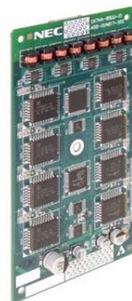
The 8-Port Analog Station Card is an expansion card that provides eight additional analog station ports. You can install up to two 8-Port Analog Station Cards, using the upper and middle expansion slots, for a system maximum of 18 analog stations.
