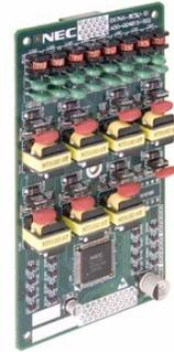
The 8-Port Digital Station Card is an expansion card that provides eight additional digital station ports. You can install up to two 8-Port Digital Station Cards, using the upper and middle expansion slots, for a system maximum of 24 digital stations.
