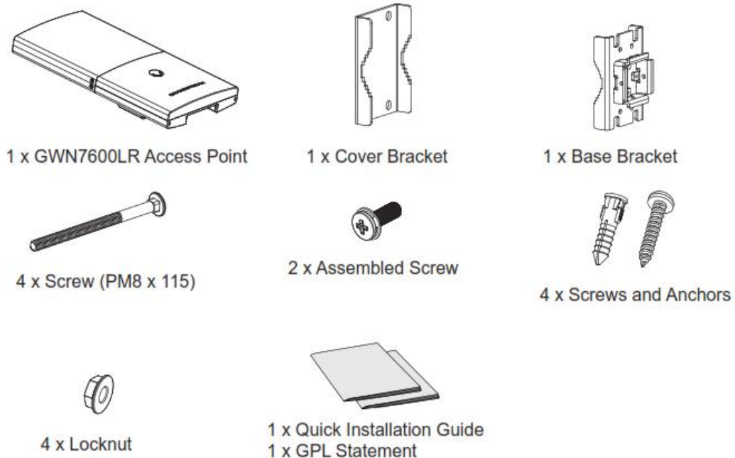
Figure 1: GWN7600LR Equipment Package
