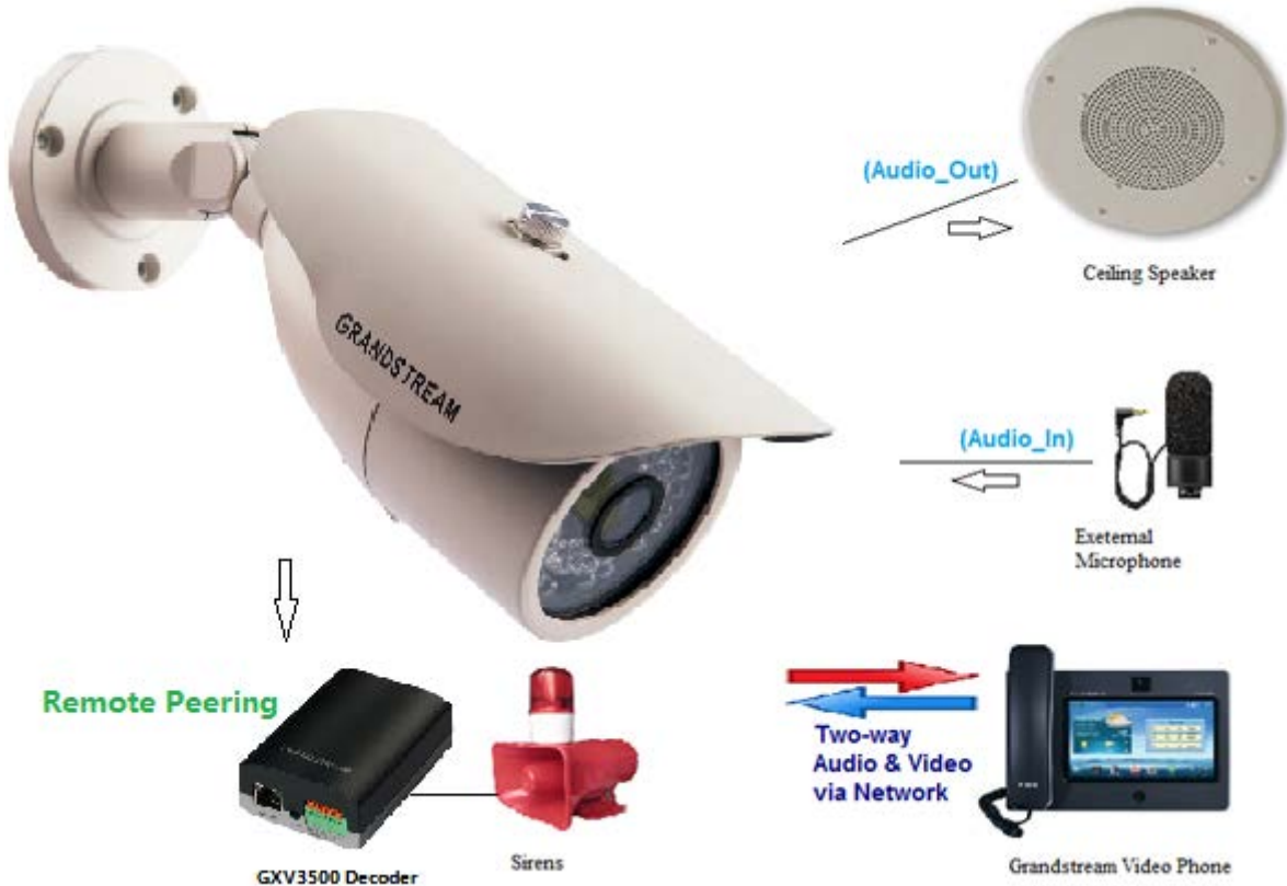
Figure 6: Application Peripheral Connection for GXV3672_HD/FHD v2
